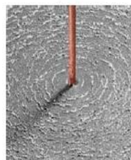
(a) A pattern of concentric circles indicating the field line of magnetic field around a straight conducting wire. The arrow in the circles show the direction of the field lines. (b) A close up of the pattern obtained.
